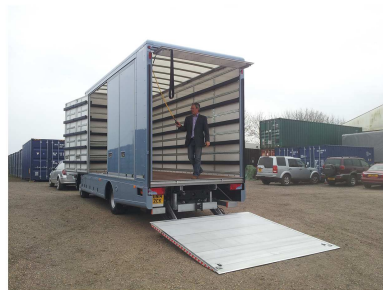
12ton box van with 2ton tailift
